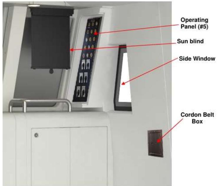
Figure 19 : Arrangement of the cab interior side right (non-Driving side)
