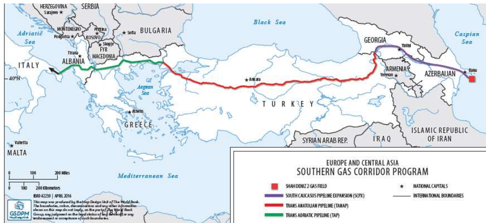
Figure 1: Route of SCPx, TANAP and TAP Pipelines from Azerbaijan to Italy
