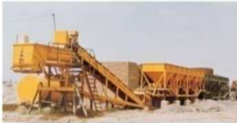
Wet Mix Plant
