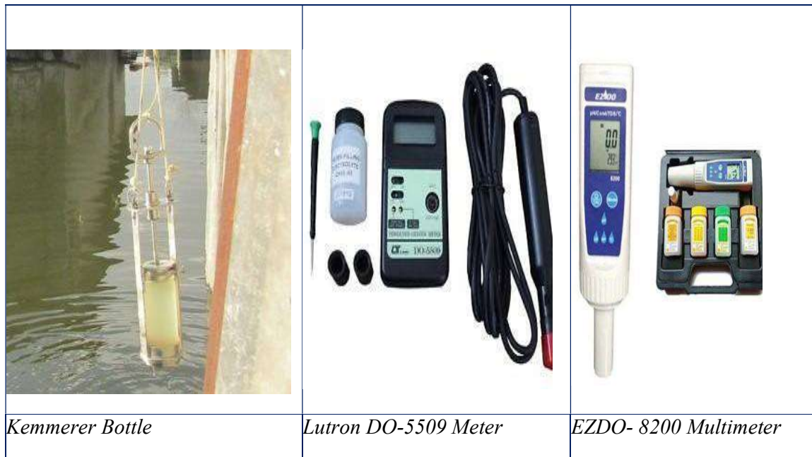
Figure 2.4 Equipment used for Surface water Sampling and On-site Testing Table 2.4 Sampling Locations of Surface Water
