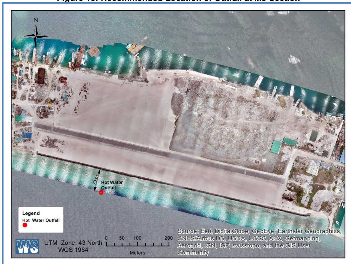
Figure 15: Recommended Location of Outfall at M8 Section
