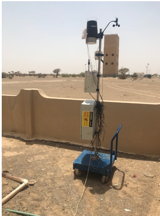
Figure 5-1 Ambient Air Quality Monitoring Station
