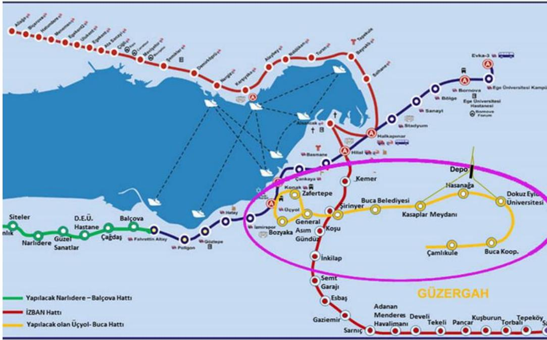
**Figure 2: Network (Navy Line) And Planned Metro Lines (Üçyol-Buca Metro Line Shown with Yellow Line, Narlidere-Balçova Metro Line Shown with Green Line), Red Line Shows the IZBAN Network**
