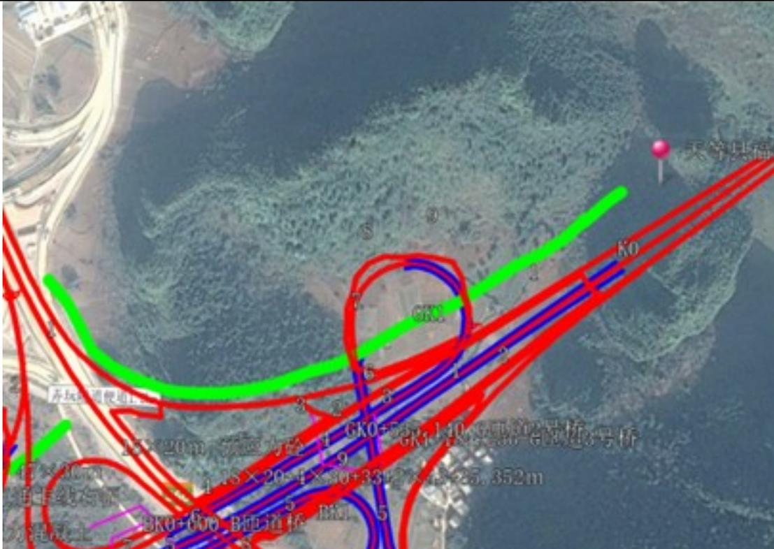
Figure 3.1-6 Location of New Access Road (1.5 km) at G Ramp
