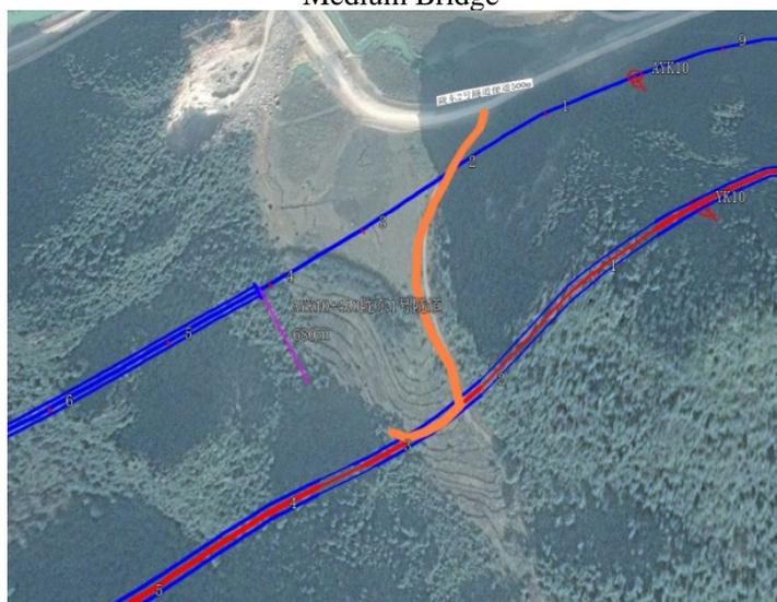
Figure 3.1-14 Location of New Access Road (500m) to Entrance of Longdong No.2 Tunnel
