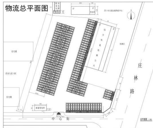
**Figure 3-9 Layout of the charging station of Yingkou Logistics Company**
