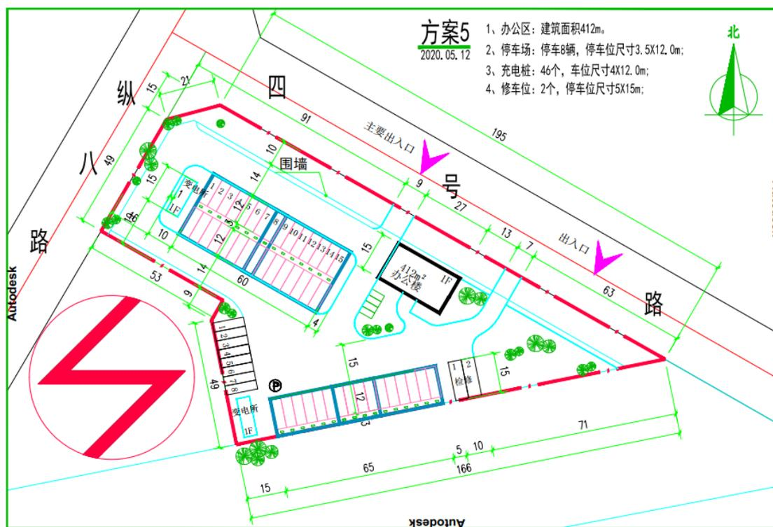
Figure 3-24 Layout of Charging Pile in Huludao Dongcheng
