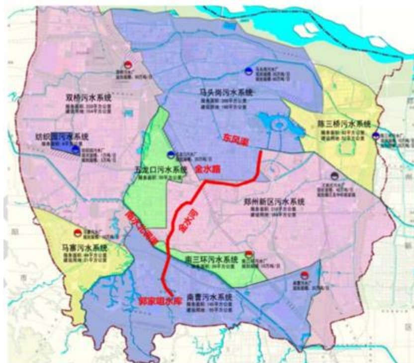
Figure 4-2 Sewage system zoning along the Jinshui River
