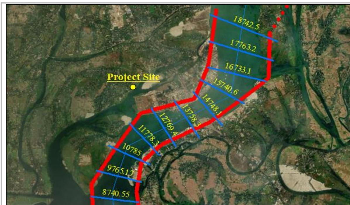
Figure 7.15: Channel in front of project site as well as its cross sections
