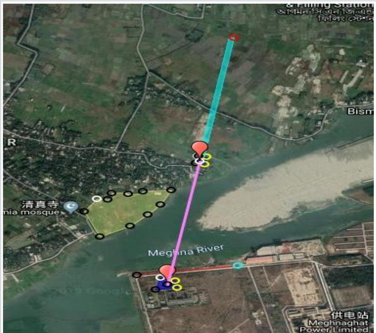
Figure 3.29: Option 4-General Layout of the Pipeline HDD
