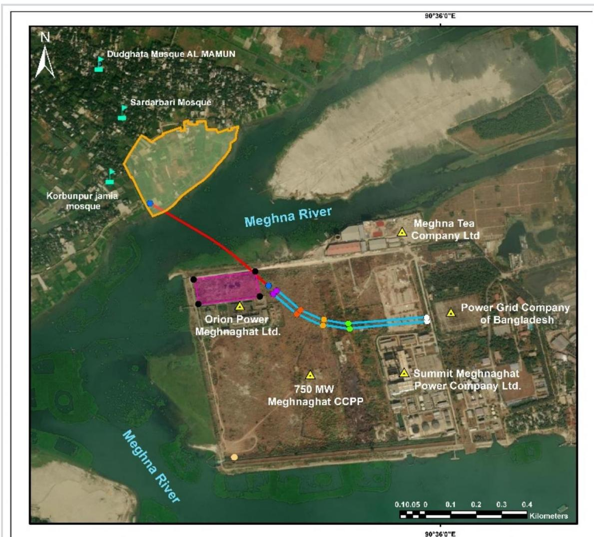
Figure 3.26: Option 1-General alignment of the Pipeline HDD
