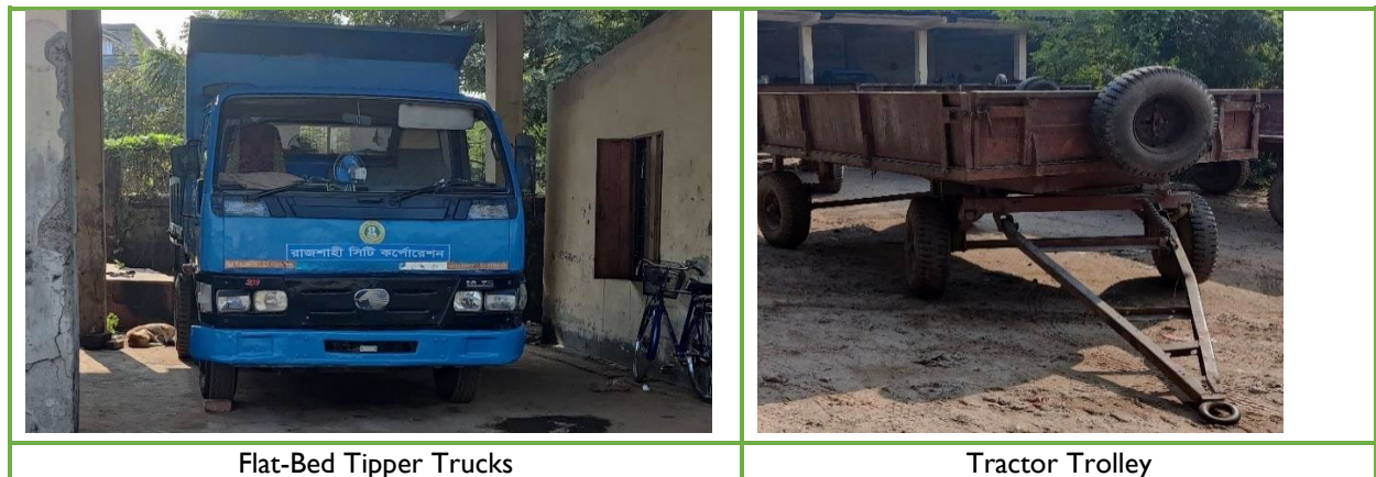
Figure 3.5 Vehicles for Secondary Waste Transportation Source: Consultant’s Team Site Visits and Field Surveys
