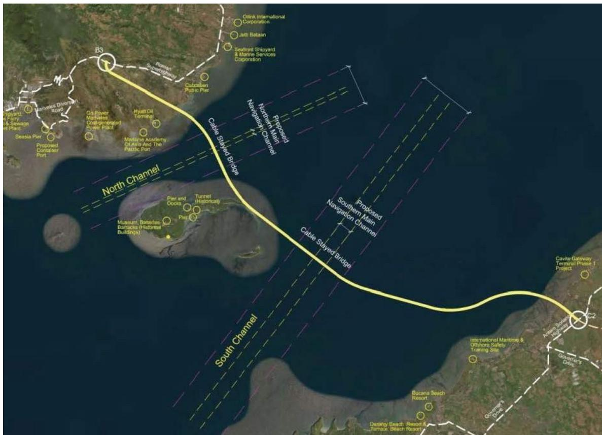
Exhibit 1 Plan View of BCIB Showing Navigation Channels
