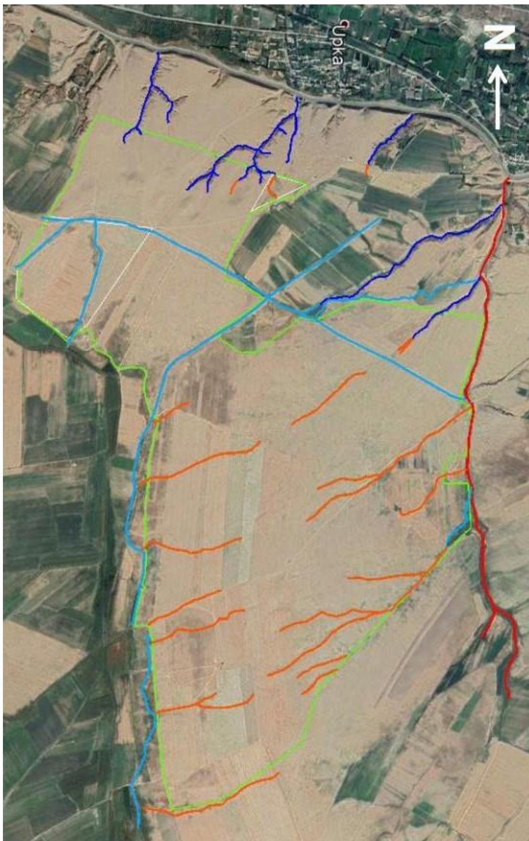
Figure 6-6 Deep gullies (blue lines), drainage ditches (light blues lines), gullies with depths less than 1.50 meters (orange lines) and a watercourse (red line).
