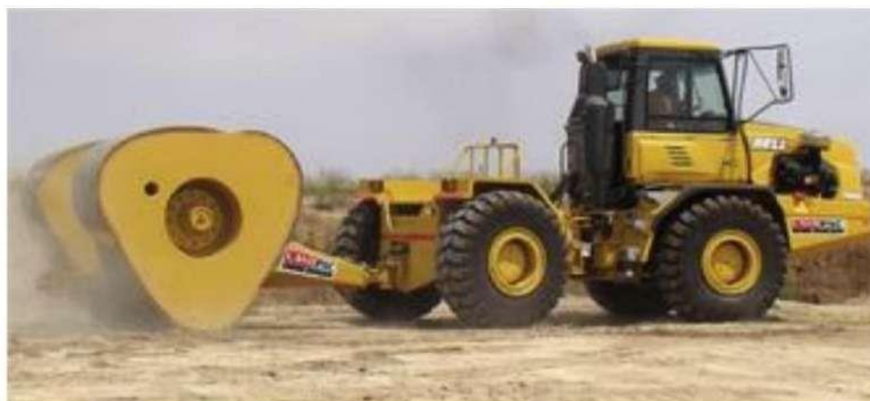
2-16 rasm. Rolling dinamik siqish (RDC)
