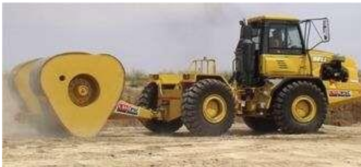
2-21-rasm. Rolling dinamik siqish (RDC)
