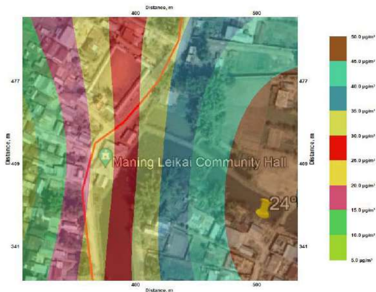
Figure 21: Isopleth for CO for the projected year 2069-70
