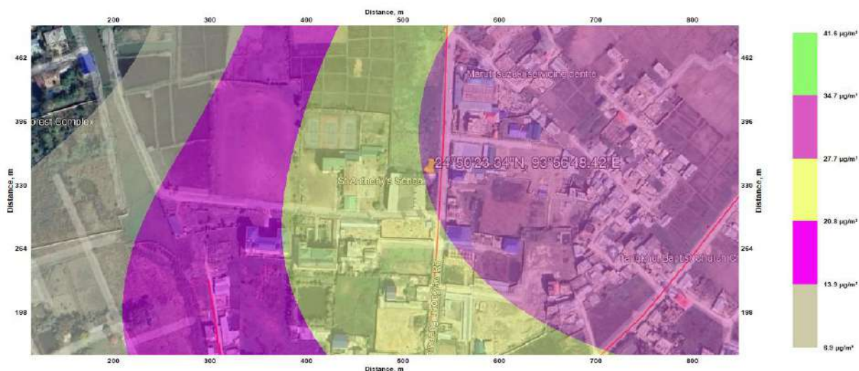
Figure 45: Isopleth for CO for the projected year 2069-70
