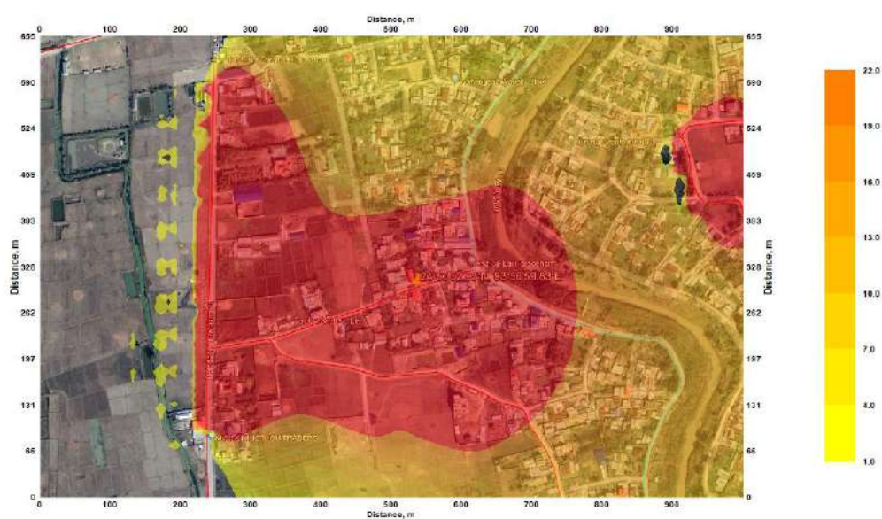
Figure 6: Isopleth for CO for the projected year 2069-70
