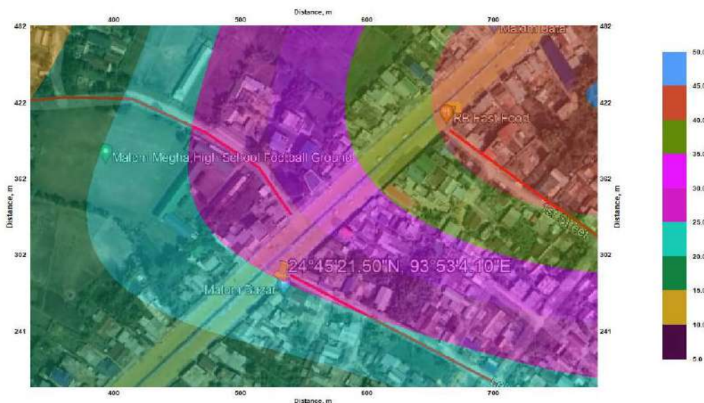
Figure 22: Isopleth for PM for the projected year 2069-70
