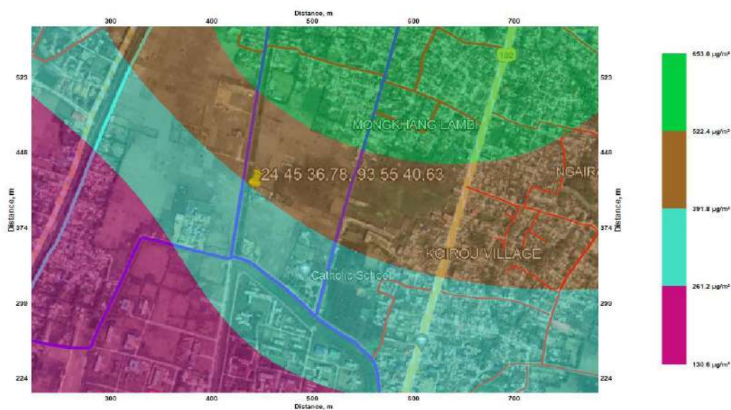
Figure 30: Isopleth for CO for the projected year 2069-70
