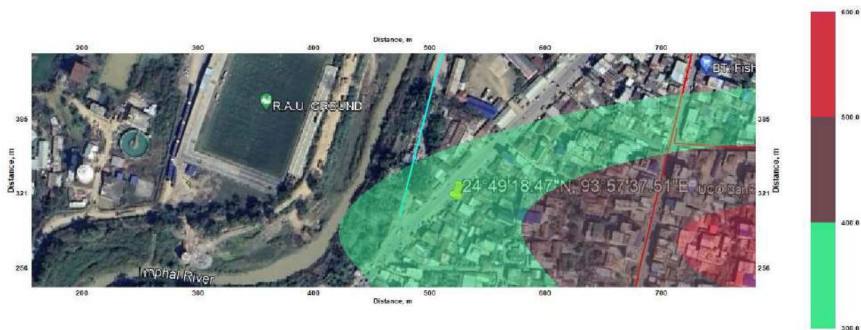
Figure 16: Isopleth for PM for the projected year 2069-70
