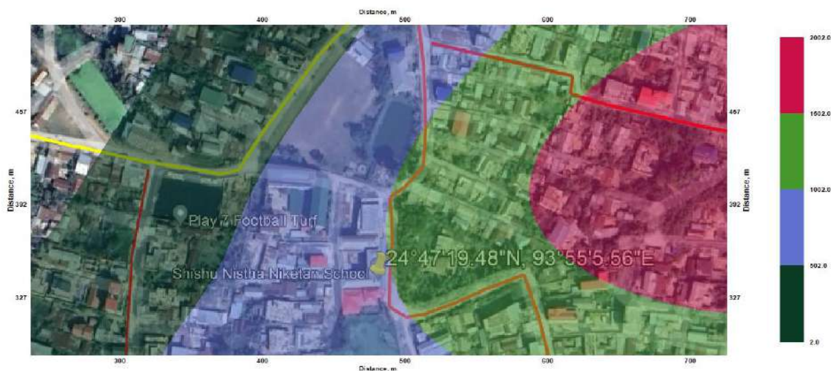
Figure 42: Isopleth for CO for the projected year 2069-70
