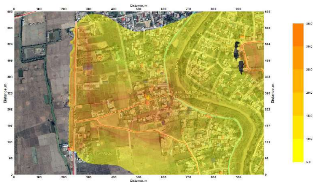
Figure 5: Isopleth for NO 2 for the projected year 2069-70
