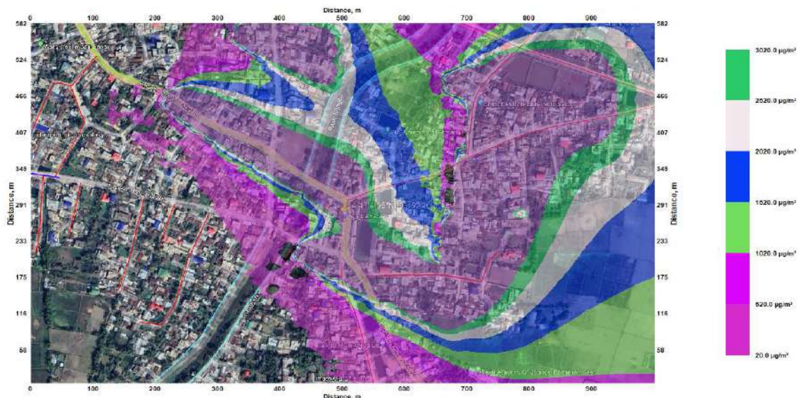
Figure 15: Isopleth for CO for the projected year 2069-70
