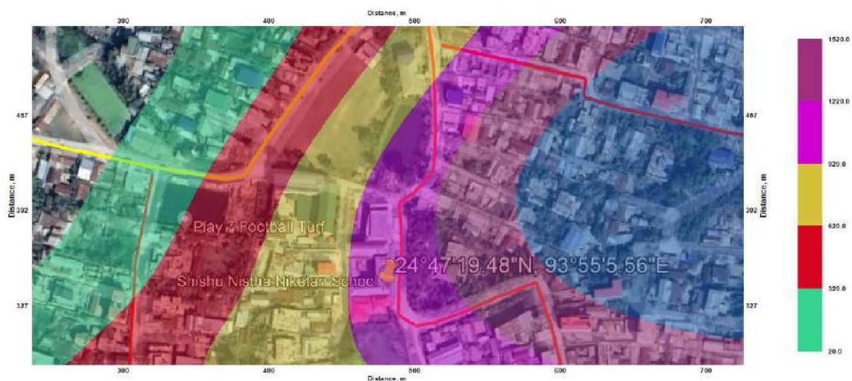
Figure 41: Isopleth for NO 2 for the projected year 2069-70
