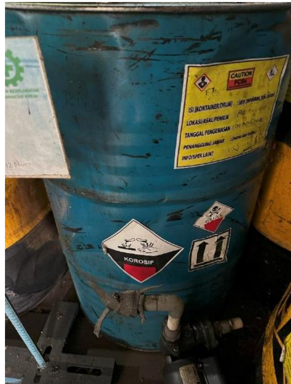
In appropriate symbols on hazardous waste packaging in Binjai warehouse in UID North Sumatra.
