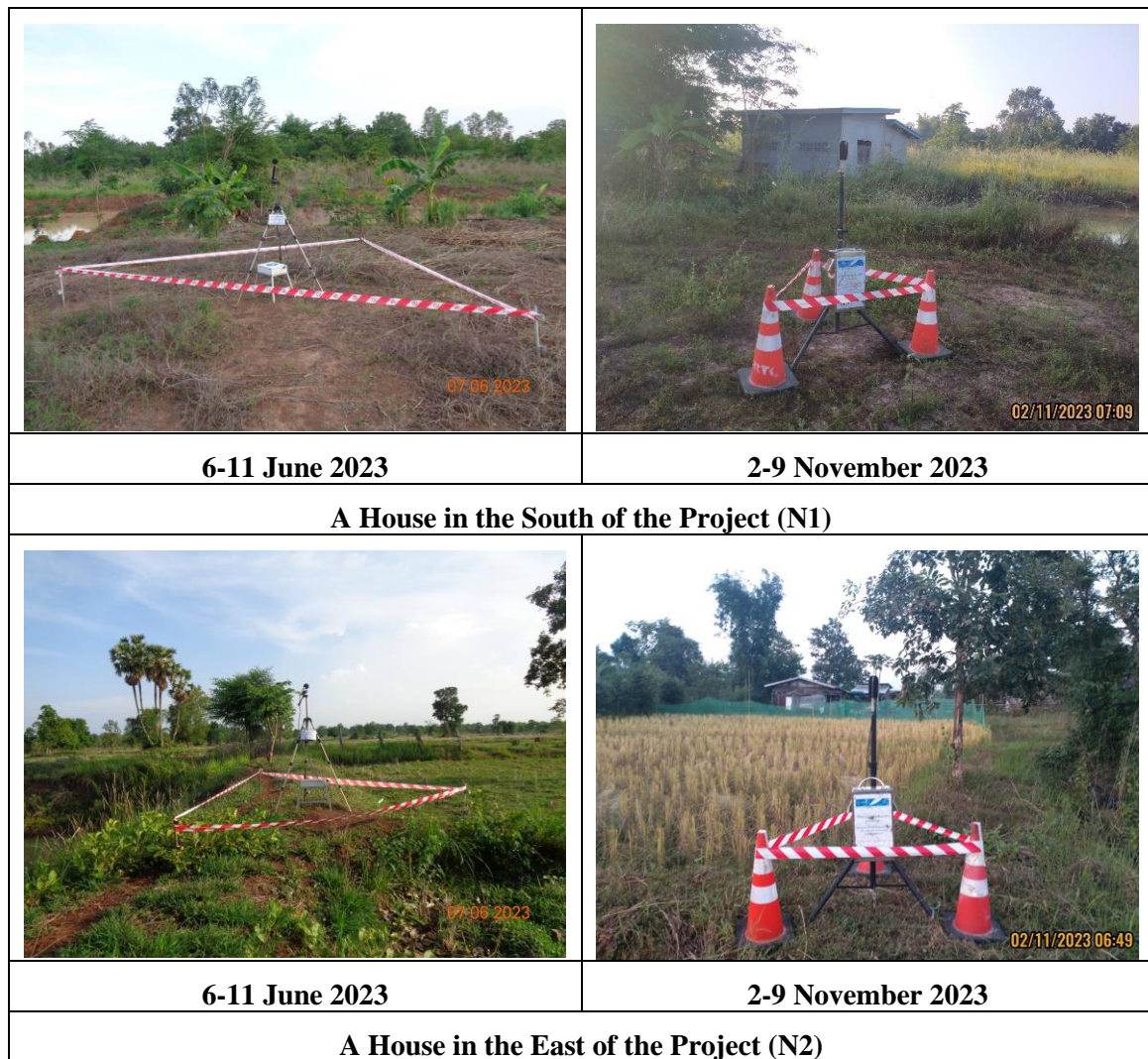
FIGURE 3.1-8 : SOUND LEVEL MEASUREMENT IN THE PROJECT AREA BETWEEN 6-11 JUNE 2023 AND 2-9 NOVEMBER 2023
